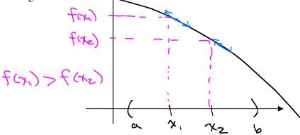
Notice that wherever a function is increasing, the tangent lines have positive slope. Notice that wherever a function is decreasing, the tangent lines have negative slope.
