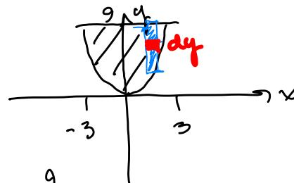
$$\begin{aligned} V &= \int_0^4 \int_{-3}^3 \int_{x^2}^9 dy dx dz \\ &= \int_0^4 \int_{-3}^3 y \Big|_{y=x^2} dy dx dz = \int_0^4 \int_{-3}^3 (9-x^2) dy dx dz = \int_0^4 \left( 9x - \frac{x^3}{3} \right) \Big|_{-3}^3 dz \\ &= \int_0^4 \left[ (9(3) - \frac{3^3}{3}) - (9(-3) - \frac{(-3)^3}{3}) \right] dz = \int_0^4 [27 - 9 + 27 - 9] dz = \int_0^4 36 dz \\ &= 36z \Big|_0^4 = 144 \end{aligned}$$
