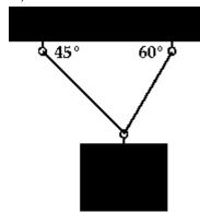
Answer: Tension in right cable: 1098.08 kg; tension in left cable: 776.46 kg
