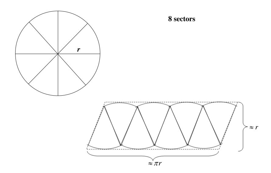
As the number of sectors increases, the assemble shape gets closer to a parallelogram with base of  $\pi r$  and a height of r, whose area is  $\pi r^2$ .
