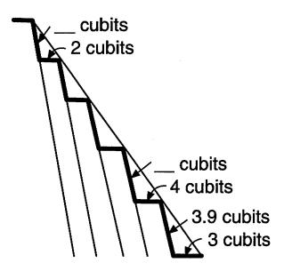
Detail from a cross section of Pyramid at Meydum (Lengths are approximate.)
