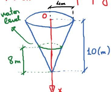
Tank: shape is an inverted come as in the picture.
