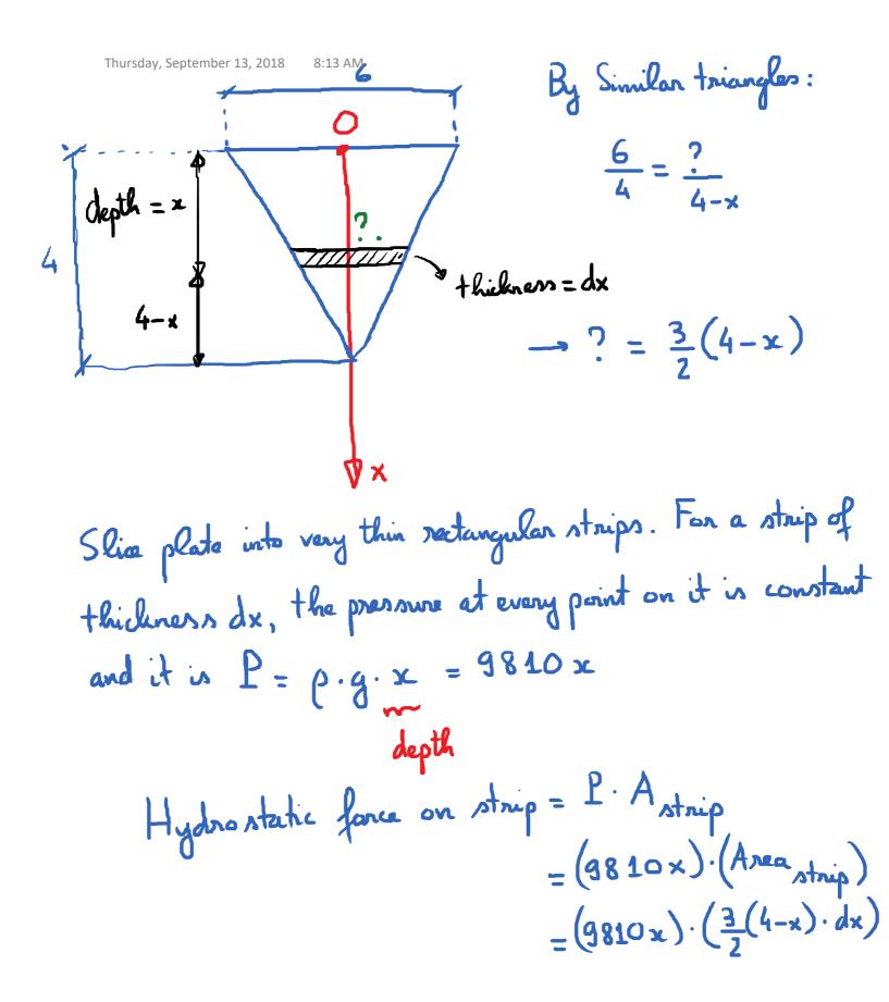
Hydrostatic force on plate = ((9810x). 3/(4-x).dx Thursday, September 13, 2018 8:22 AM water surface Ex. depth 6m  $x^2 + y^2 = 4$ 8m hickness = dy Set up the integral to find the hydrostatic force acting on this incular plate. 9810(8-y) Pressure strip = p.g. (8-y) = Force strip = L'strip Astrip = 9810(8-y).(214-y²) dy
