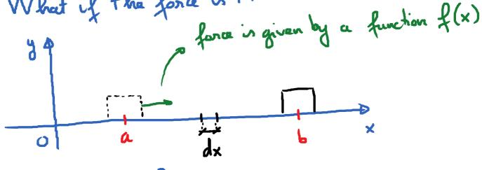
Divide the distance from a to b into really small segments dx. We can consider the force to be constant within each such small regment.
