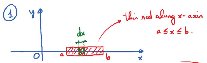
Density at a point x is given by the function p(x)
